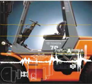
The new series uses a full-floating system that vastly reduces the amount of engine vibration transmitted to the frame, assuring a ride of unmatched comfort. This promises not only more comfort for the operator, but greater frame durability as well.
